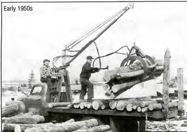
The first hydraulic loader built in Leo Heikkinen's shop, undergoing field trials. Leo (on truck cab) is working the controls and Al Swan (on load bed) is getting the load lined up to be lowered in place.
