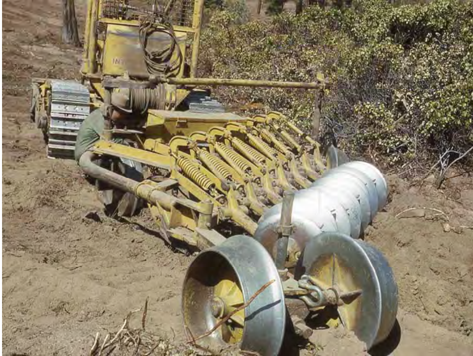
Rangeland plow used for site preparation, Goosenest Ranger District, Klamath National Forest, 1965.
