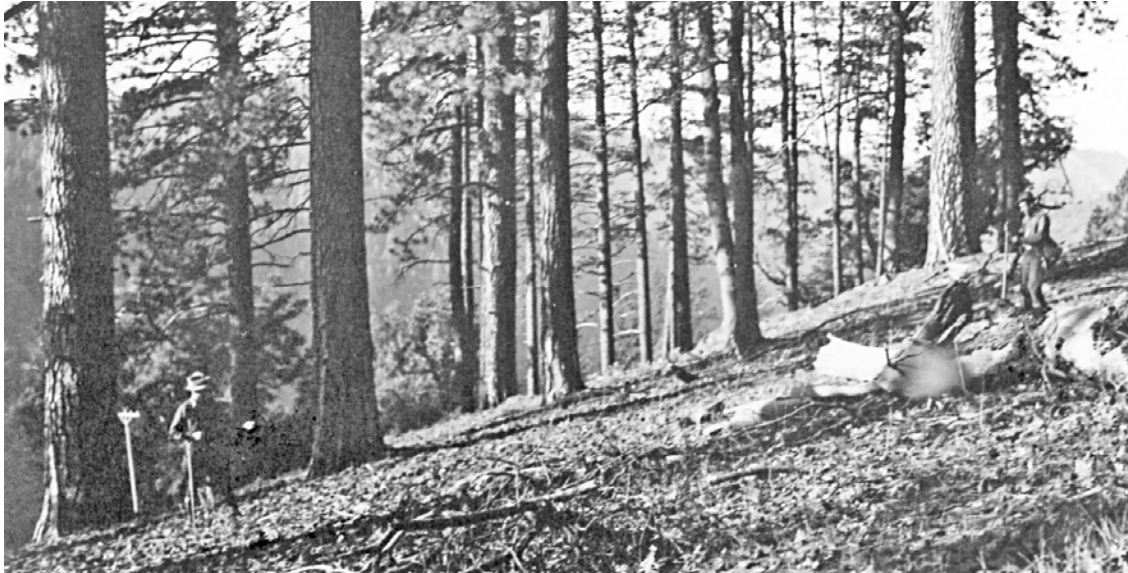
Chaining on a slope with Abney and 2 ½ chain topographic trailer tape, Prather Creek cruise, Eldorado National Forest, 1935.
