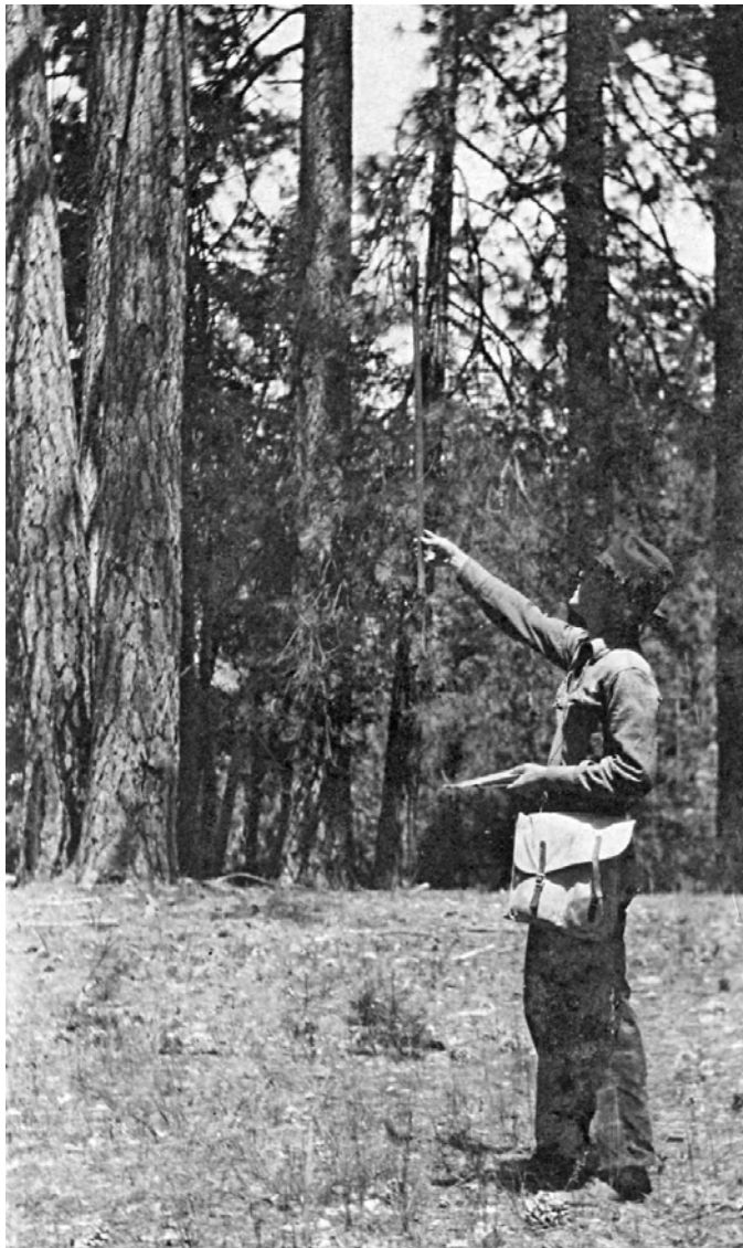
Oscar Evans using the Biltmore stick hypsometer to estimate tree height in 16-foot logs to an 8-inch merchantable top, the Eldorado Project, 1923.
