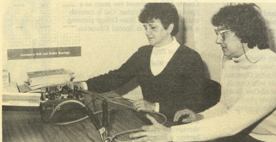
Virginia Beacom, Quality Control Supervisor, demonstrates for Joyce Fonti, Workshop employee, the use of a testing meter used to test the electrical resistance of each ground rod produced.
