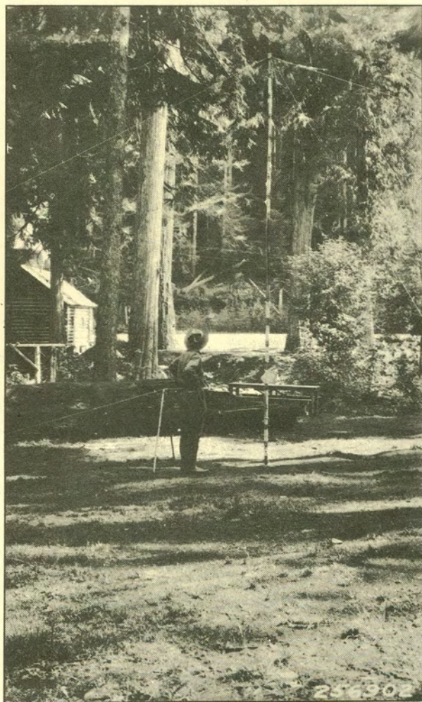
A test station located near Rainier National Park. Antenna pole and counterpoise support in foreground.
