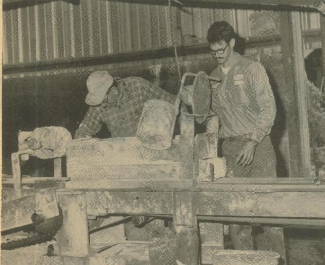
CARL STIMPSON, AND Bart Jennings, III, tending "heart" machine of the industry. Along a conveyor the clay goes into a pug mill and vacuum chamber from which it is extruded in a solid column to a cutter where 18 bricks are cut at one time. (Photo by Keith Wood)
