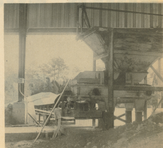
THE CLAY IS FED into this hopper after which it goes through an apron feeder where it undergoes three more grindings. (Photo by Keith Wood)
