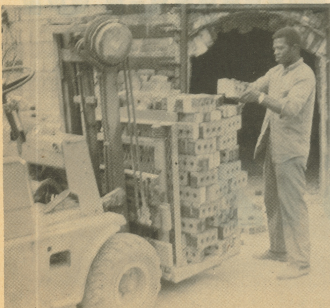
WILLIAM HOLLINGER shown unloading bricks from kiln onto fork lift. (Photo by Kay Nuzum)
