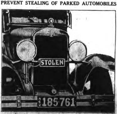
The new device which blazes out the word, "Stolen," directly when a thief attempts to switch on the ignition of a parked motor car, in an attempt to steal it. The secret of the new device lies in a little box attached to the ignition system which it is necessary to unlock before the ignition is switched on. The invention is pronounced absolutely infallible.
